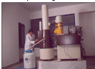
Liquid Nitrogen Plant
